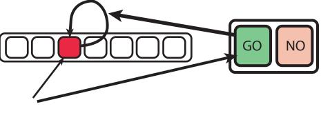
Inputs project to both the stripe and the gate. If the input activates the GO unit, the current self connection is removed, allowing the new input to gain access to the stripe. The input then activates the GO unit again, which locks the new input.
